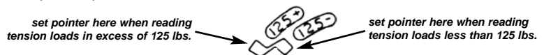
Figure 2. Pre-set Instructions for type C-8 Instrument. For type C-9 Instruments, use Similar Procedure
